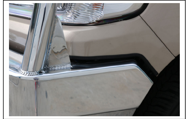
Figure 10 : 3mm clip lock, trimmed to suit rear of cut.
